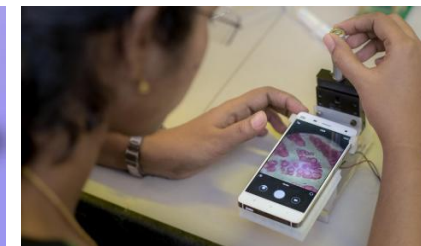
Low-cost lenses to turn smart phones into microscopes
