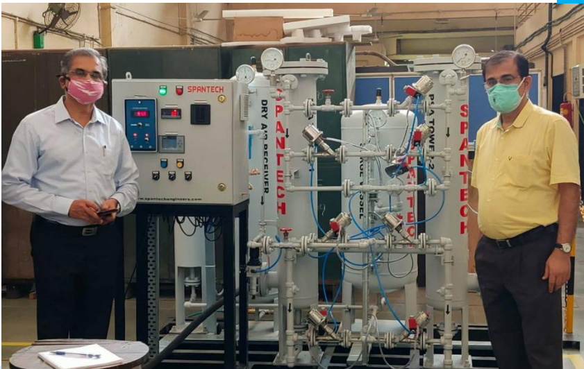
Indigenous system to produce oxygen from nitrogen generator
