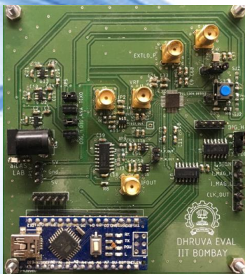
Dhruva: Indian RF receiver chip for NAVIC & GPS Satellites
