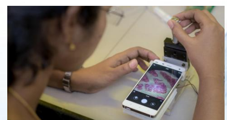
Low-cost lenses to turn smart phones into microscopes
